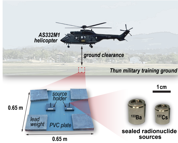
Figure 5: Experimental setup of the far-field radiation measurements. The main elements of the setup are the fully integrated Swiss AGRS system operated in hover flight mode at a predefined ground clearance above a sealed radionuclide point source positioned on the ground in a custom source holder. Two different sources have been deployed separately: a ^{137}\text{Cs} source ( \mathcal{A} = 9.0(5) \times 10^9 Bq) and a ^{133}\text{Ba} source ( \mathcal{A} = 4.7(2) \times 10^8 Bq). The source holder consisted of a polyvinyl chloride (PVC) base plate with two custom source holders made from polylactide polymer (PLA) and constructed using additive manufacturing techniques. The base plate was secured to the ground using four lead bricks, each with a mass of 11.3 kg. Note that the adopted zoom-in figures of the radionuclide sources are only representative of their size and geometry and do not depict the actual sources deployed during the measurements.
