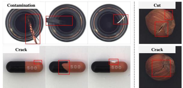
**Fig. 2.** Examples of ambiguous defect category definitions from MVTEC AD [19]. The defects in the left part exhibit clear pattern differences, yet they are assigned to the same categories. Instead, the defects in the right part appear similar, but they are classified into different categories.
