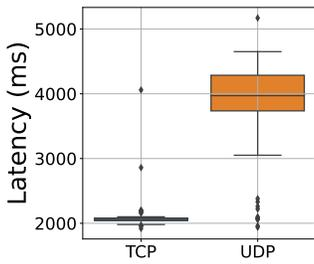
Figure 7: *SMBHYB\_rem* TCP vs UDP auth. latency.
