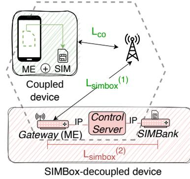
**Figure 4: Signaling latency of coupled and SIMBox-decoupled devices.**
