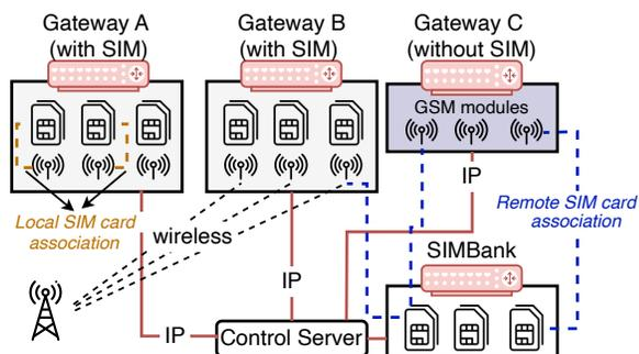
Figure 2: Example of a *SIMBox* distributed architecture.
