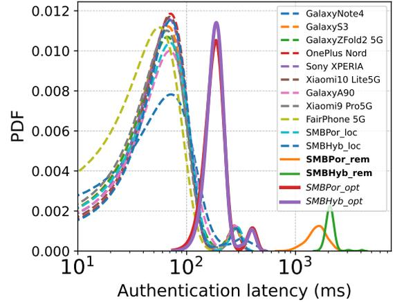
**Figure 13: Distribution of authentication latency of (i) coupled devices (*dashed*), (ii) current (*bold label*) and (iii) optimized (*italic label*) *SIMBox*-decoupled devices**
