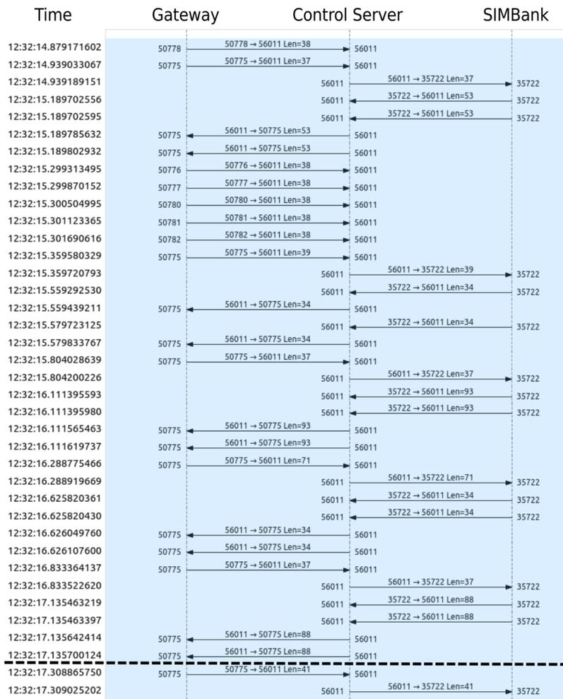
Figure 17: Hybertone SIMBox components UDP interactions during authentication
