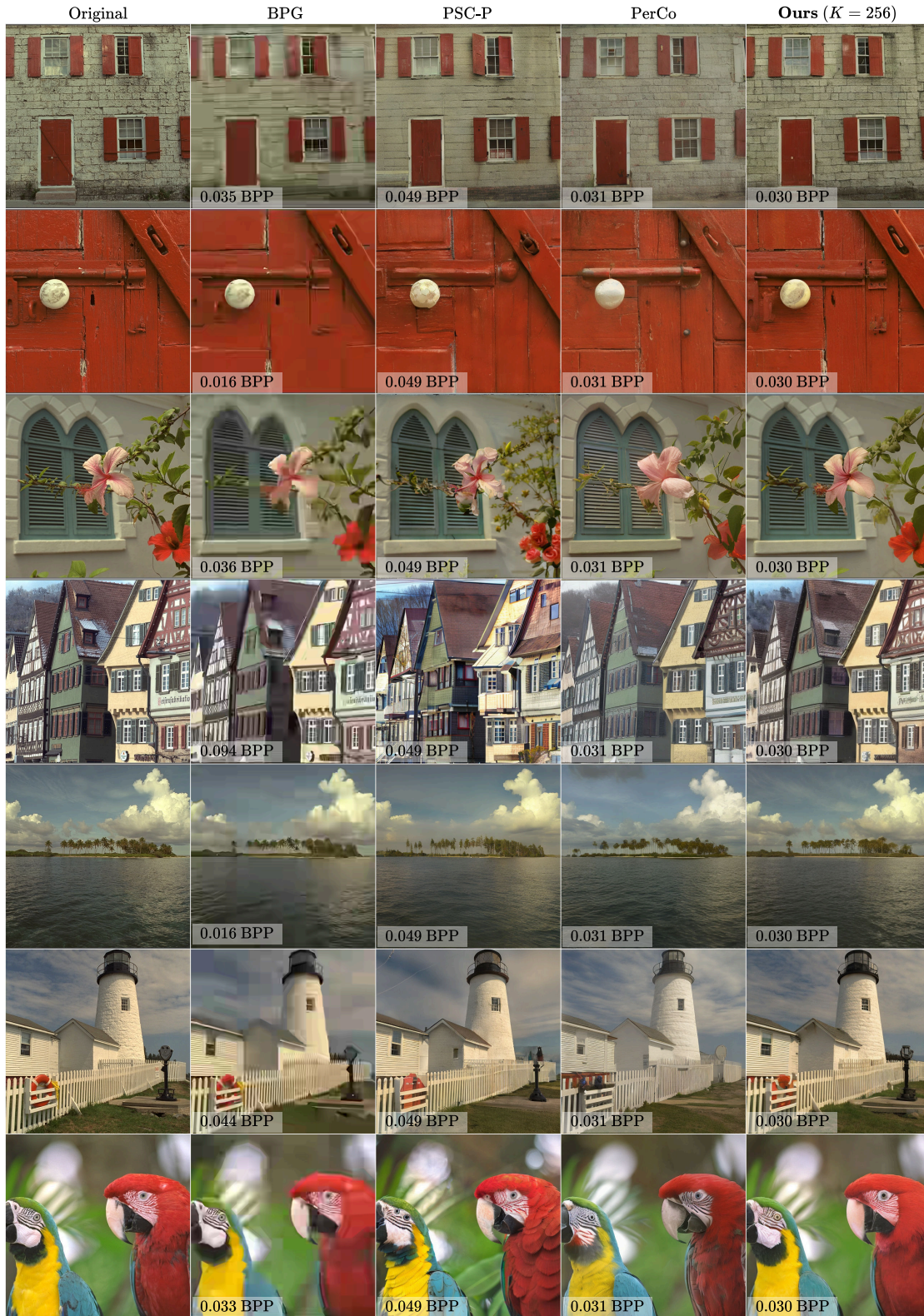
Figure 11. Qualitative extreme image compression results. The presented images are taken from the Kodak24 dataset, cropped to 512 \times 512 pixels. Our compression scheme produces highly realistic decompressed outputs, while maintaining better fidelity to the original images compared to previous methods.
