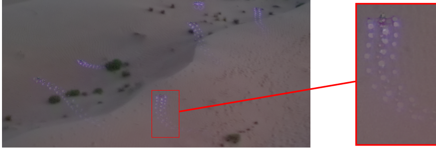
Figure 1: Six agile swarm members flying in challenging desert conditions, relying on UVDAR-based relative localization as used in this work.
