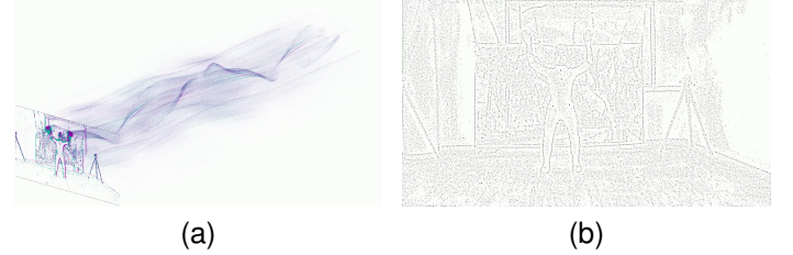
Fig. 5. Example surface using the EROS algorithm to enable velocity-independent representation without temporal parameter tuning: (a) the input events over time for an example scene, (b) a visualization of the EROS surface after integrating event information over the entire time period of the dataset.
