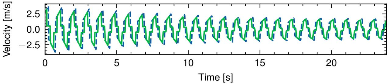
Fig. 6 Velocity for copper slurry on 2 control points, at  $x = 0$  (blue) and  $x = L/2$  (green)
