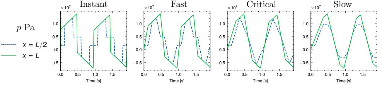
**Fig. 12** Valve closure time impact on pressure evolution
