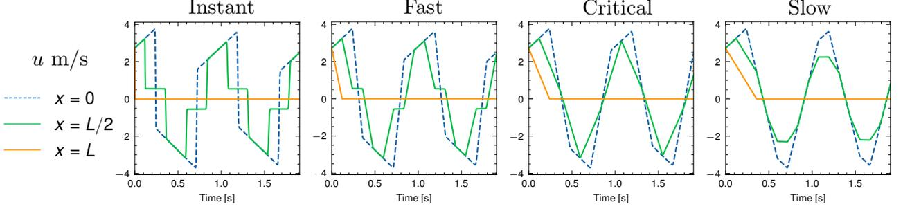
**Fig. 11** Valve closure time impact on velocity evolution
