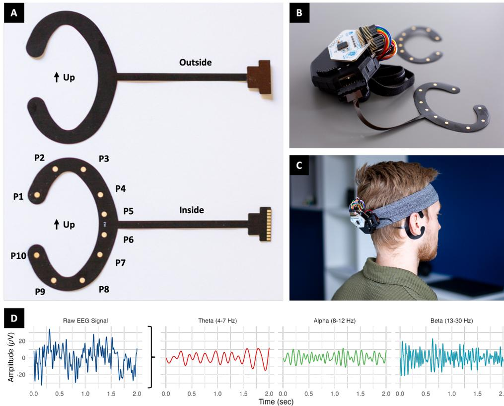
Fig. 2. Gold-plated open-cEEGrids (A) together with OpenBCI Cyton+Daisy 16-channel biosignal amplifiers (B), worn by a study participant (C), and with examples of one channel's signals with decomposed frequency bands (D).
