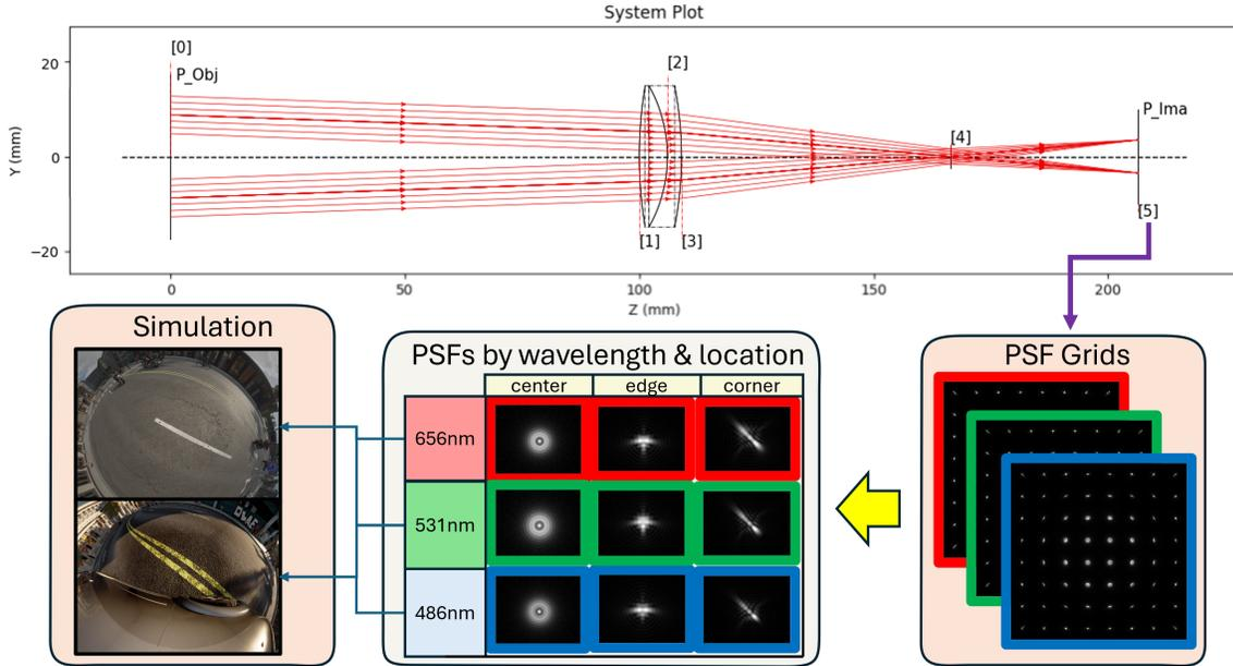
Figure 1: *Degradation Pipeline of an Optical Doublet where all surfaces are labeled between [0-5] with ray-tracing performed between  $\pm 2^\circ$  FOV and light wavelengths of  $w = (656nm, 531nm, 486nm)$  (red, green, blue). The generated PSF grid outputs are then convolved with two simulation images.*
