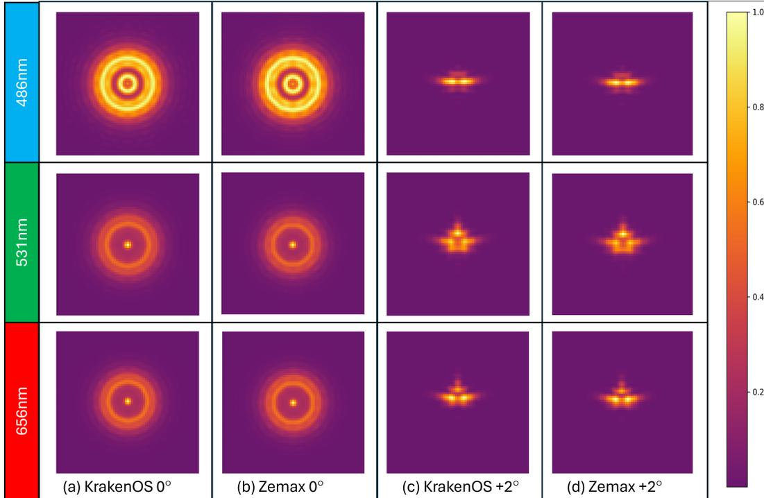
Figure 3: *Fraunhofer Point Spread Functions at 0° and +2° FOV where  $w \in [486nm, 531nm, 656nm]$*
