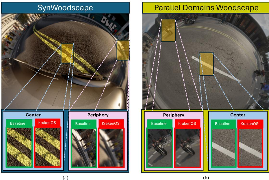
Figure 4: *Optical degradations of both (a) SynWoodscape and (b) Parallel Domain Woodscape where green frames represent the baseline cases with no degradations applied and red frames represent degraded cases after convolving the test images with KrakenOS.*
