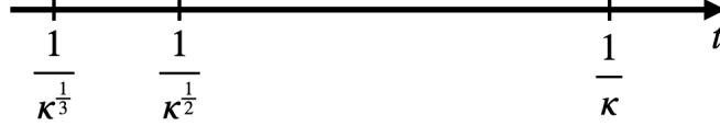
FIGURE 3. Comparison between the pure diffusion time scale t \sim \frac{1}{\kappa} and the enhanced dissipation time scales in the case of a monotone shear flow t \sim \frac{1}{\kappa^{\frac{1}{3}}} and one admitting simple critical points t \sim \frac{1}{\kappa^{\frac{1}{2}}} .
