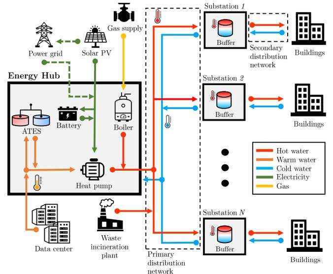
Fig. 1. A schematic diagram of a district heating network with multiple substations (consumers) and production points.
