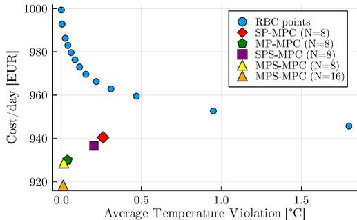
(a) Daily operating costs versus temperature violations for a DHN with sufficient pumping capacity.
