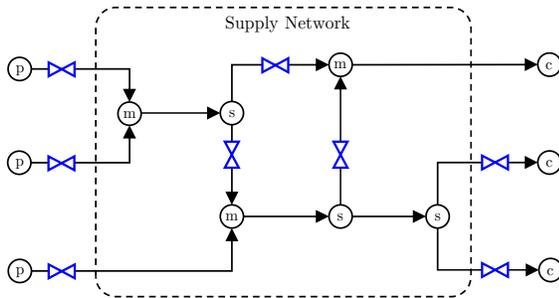
Fig. 4. The valve checking procedure, described in Remark 4, illustrated by showing the flow from producers (p) to consumers (c) going through the supply network consisting of merging nodes (m) and splitting nodes (s).
