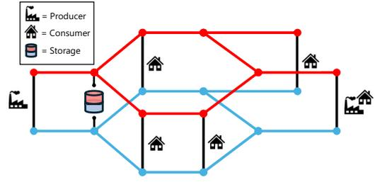
Fig. 2. The AROMA district heating network with multiple consumers, a prosumer, a storage buffer, and a loop.
