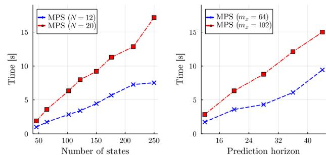
Fig. 15. The left figure shows median solver times for the MPS-MPC algorithm using a prediction horizon  $N = 12$  and  $N = 20$  for different number of state variables. The right figure shows for two models, one with 64 states and one with 102 states, the median solver time based on the chosen prediction horizon.
