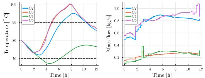
Fig. 13. Consumer inlet temperatures and mass flows for a single-producer (SP-MPC) case.
