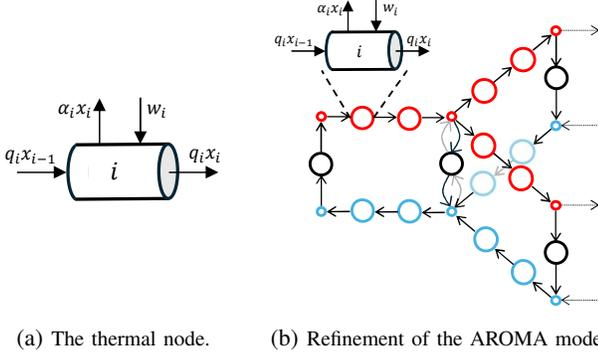
Fig. 5. Illustration of thermal node model and mesh refinement of the DHN graph. (a) shows the conceptual thermal node model with its dynamics defined by (41), while (b) demonstrates the injection of thermal nodes in a section of the AROMA network.
