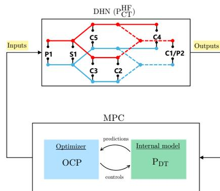
Fig. 8. The block diagram showing the MPC feedback scheme.
