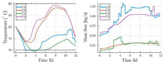
Fig. 14. Consumer inlet temperatures and mass flows for a multi-producer (MP-MPC) case.
