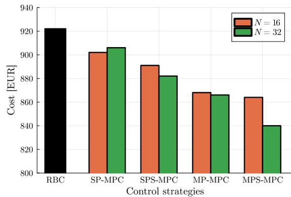
Fig. 10. Results of simulation 1. All results are based on 24 hours of simulation. Results from left to right are for: rule-based control (RBC), single-producer MPC (SP-MPC), single-producer MPC with storage (SPS-MPC), multi-producer MPC (MP-MPC), and multi-producer MPC with storage (MPS-MPC). The average runtime for each iteration of the MPC algorithms was under 10 seconds.
