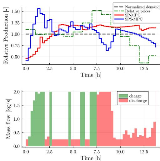
Fig. 12. The top figure shows the power injected into the network relative to the demand being extracted for both the SP-MPC and the SPS-MPC methods. The green line denotes the normalized cost of generating heat and is shown for reference. The bottom figure shows the charging and discharging modes of the storage buffer in the SPS-MPC. For comparison the net mass flow entering or leaving the storage is equal to zero for the duration of the simulation.
