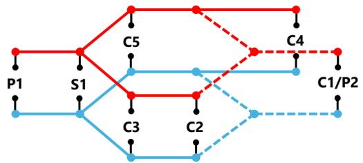
Fig. 7. The AROMA network labeled with five consumers (labeled C), two producers (labeled P), and a storage (labeled S). Dashed lines indicate pipes on which bidirectional flows are allowed.
