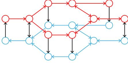
Fig. 3. A directed graph abstraction of the AROMA district heating network with fixed flow directions. Double-sided arrows indicate two opposite facing edges.
