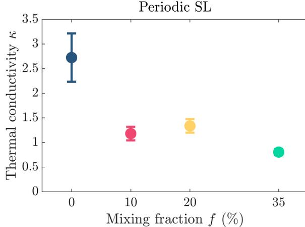
FIG. 3. Cross-plane thermal conductivity  $\kappa$  (at 30 K) versus mixing fraction  $f$  for 8 period periodic SL supercells computed from EMD simulations.  $\kappa$  is evaluated with Eqn. 4.
