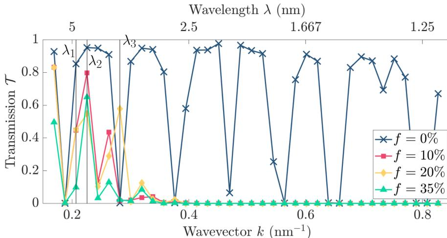
FIG. 2. Transmission  $\mathcal{T}$  versus wavevector  $k$  (or inverse of wavelength  $\lambda$ ) for the LA-mode incoherent phonon wave-packet propagating through periodic SL devices of differing mixing fractions  $f$  as shown in Fig. 1a.  $\mathcal{T}$  is evaluated with Eqn. 3. Key wavelengths  $\lambda_1 = 4.84$  nm,  $\lambda_2 = 4.43$  nm, and  $\lambda_3 = 3.55$  nm analyzed in this paper are indicated by the vertical black lines in the figure.
