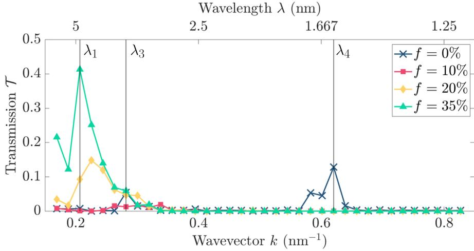
FIG. 4. Transmission  $\mathcal{T}$  versus wavevector  $k$  (or inverse of wavelength  $\lambda$ ) for the LA-mode incoherent phonon wave-packet propagating through aperiodic SL devices of differing mixing fractions  $f$  as shown in Fig. 1b.  $\mathcal{T}$  is evaluated with Eqn. 3. Key wavelengths  $\lambda_1 = 4.84$  nm,  $\lambda_3 = 3.55$  nm, and  $\lambda_4 = 1.61$  nm analyzed in this paper are indicated by the vertical black lines in the figure.
