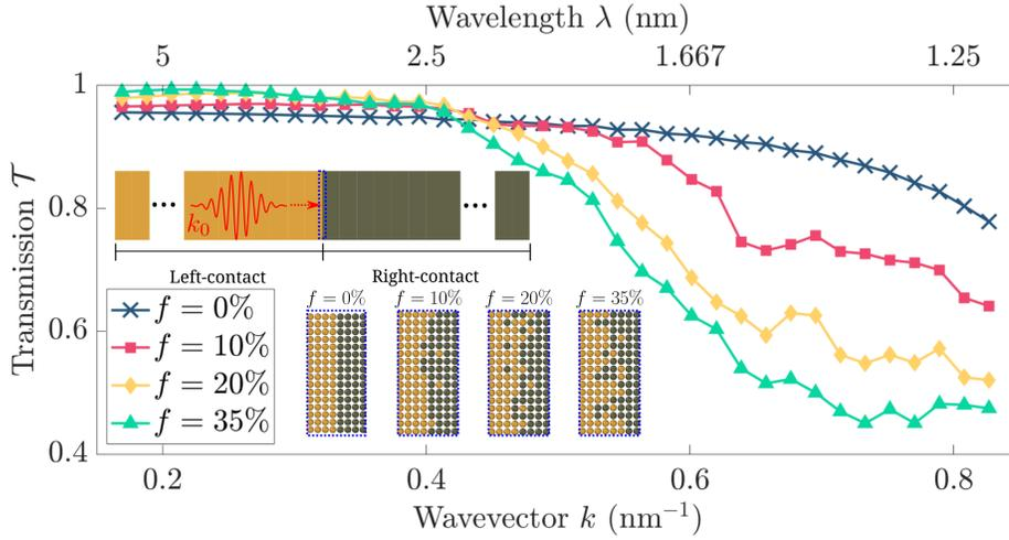
FIG. 8. Transmission  $\mathcal{T}$  versus wavevector  $k$  (or inverse of wavelength  $\lambda$ ) for the LA-mode incoherent phonon wave-packet propagating across a single m40-m90 interface of differing mixing fractions  $f$  as shown in the schematic illustration inset.  $\mathcal{T}$  is evaluated with Eqn. 3.
