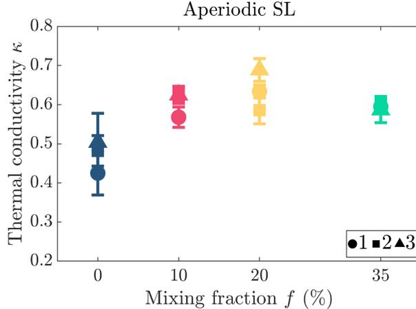
FIG. 5. Cross-plane thermal conductivity  $\kappa$  versus mixing fraction  $f$  for 8 period aperiodic SL supercells computed from EMD simulations.  $\kappa$  is evaluated with Eqn. 4. The circle, square, and triangle data points delineate the values for three different aperiodic patterns.
