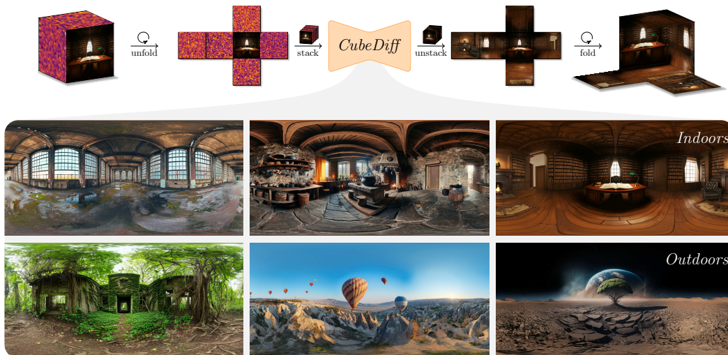
Figure 1: CubeDiff leverages cubemaps to represent 360° panoramas and denoises all faces together in a single pass. In contrast to other works, Cubediff does not need to consider distortions, since it operates on common 90° FOV perspective images, making it possible to directly utilize the internet-scale image prior of the underlying diffusion model.
