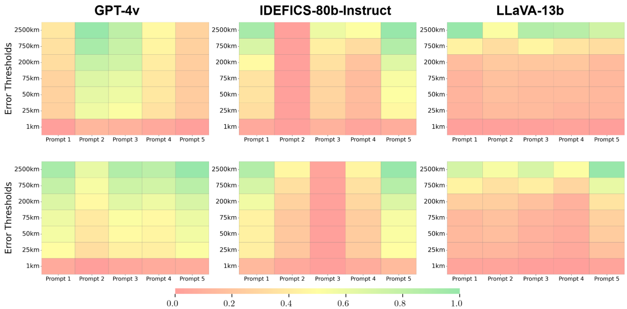
Fig. 6. Impact of prompt formulation and variation on geo-localization performance. Single-sentence prompts (top row) exhibit significant variability and lower accuracy, while structured LTM prompts (bottom row) improve overall performance and consistency. However, even with the added structure of LTM prompts, performance remains sensitive to semantically equivalent variations in phrasing.
