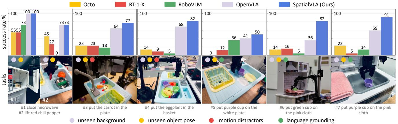
Fig. 5: **Zero-shot Robot Control Evaluation on WidowX Robot.** We evaluate SpatialVLA across 7 task suites to explore the language grounding, semantic understanding, and motion sensing capabilities, with varying backgrounds, poses, and motion distractors. SpatialVLA achieves the highest average success rate, outperforming all generalist manipulation policies.
