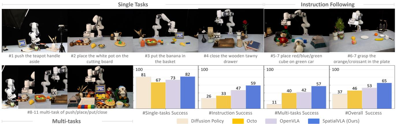
Fig. 6: **Adapting to New Robot Setups on Franka Robot.** SpatialVLA serves as a generalist robot control policy, achieving better performance across multiple setups, and can be effectively used as an initialization for fine-tuning to new robot tasks.
