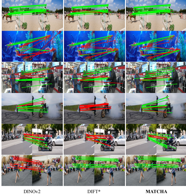
Figure 5. Visualization of temporal matches on TapVID-Davis [12]. Here we visualize several challenging cases for establishing temporal correspondences, where MATCHA generally achieves the best performance in handling extreme scale and viewpoint changes, as well as scenes with multiple similar instances. (DIFT* is the adapted DIFT where we use its concatenated semantic and geometric feature for temporal matching for better performance. )
