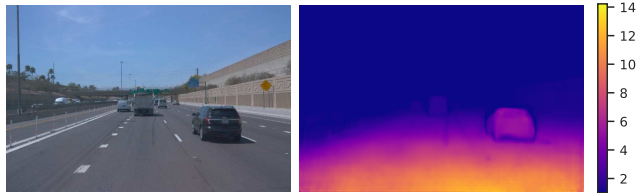
Figure 6. Global confidence map (right) produced by Light3R-SfM for an image of a sequence containing dynamic objects (left).
