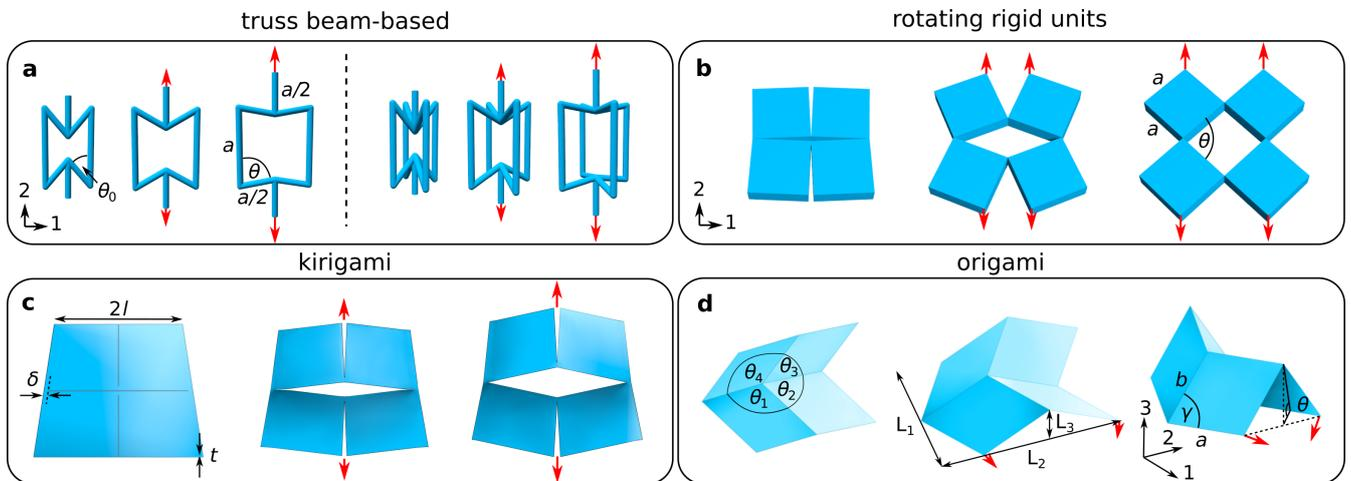
Figure 3: **Unit cells based on internal rotations.** Panels show unit cells made from **a** rods, **b** rotating blocks, **c** kirigami and **d** origami that can be used to assemble larger rotation-based shape morphing metamaterials. Red arrows on all panels indicate the applied loading.
