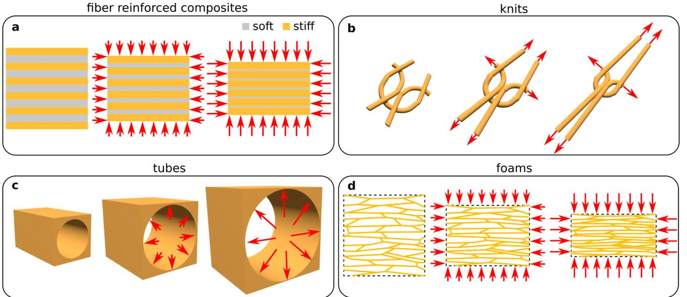
Figure 1: **Unit cells based on anisotropic mechanism.** Panels show anisotropic unit cells made from **a** fiber-reinforced composites, **b** knits (adapted from [29]), **c** pneumatic tubes and **d** foams that can be used to assemble larger anisotropy-based metamaterials. Red arrows on all panels indicate the applied loading.
