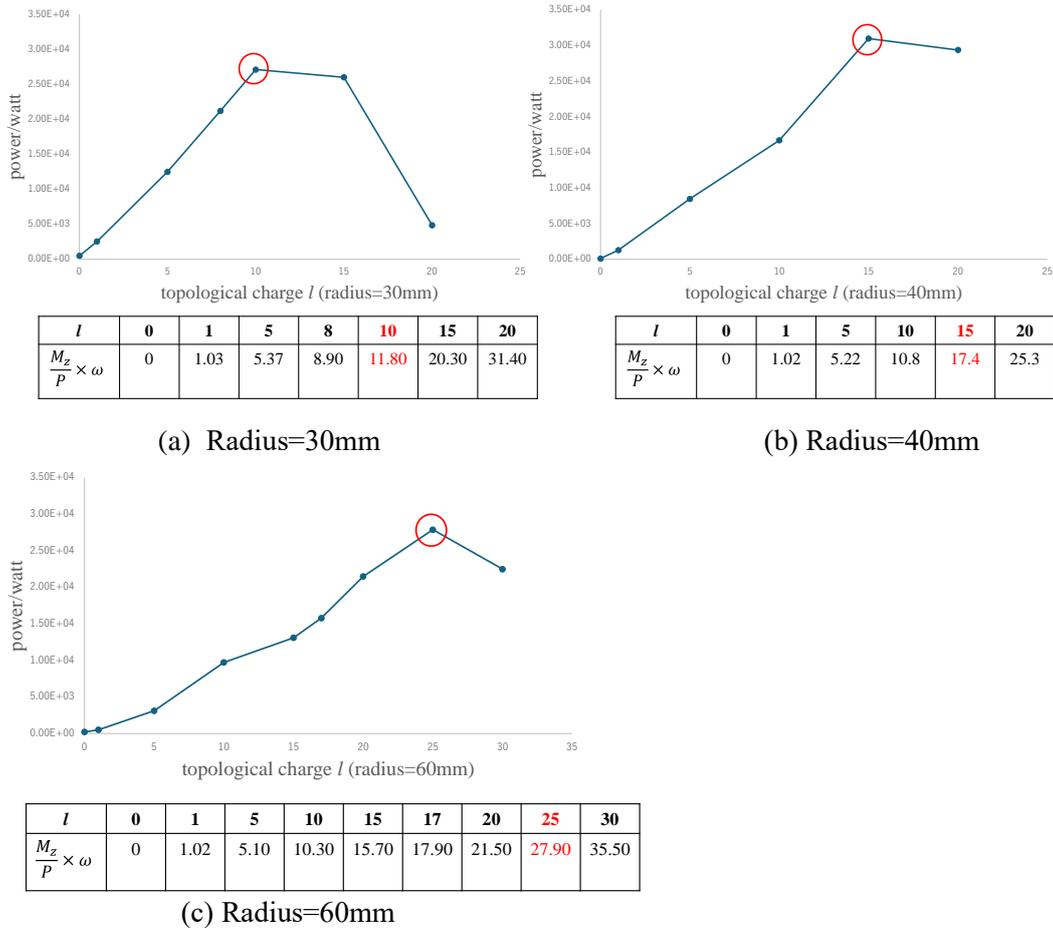
Figure 3: Propagation power of vortex fields in plasma for topological charge  $l$
