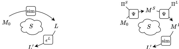
(a) Synthetic process data generation methods (b) Generation of synthetic process data with behavioral and recording deviation patterns  $\Pi^S$  and  $\Pi^L$  and model transformation function  $\Psi$  with noise injection function  $\epsilon^L$
