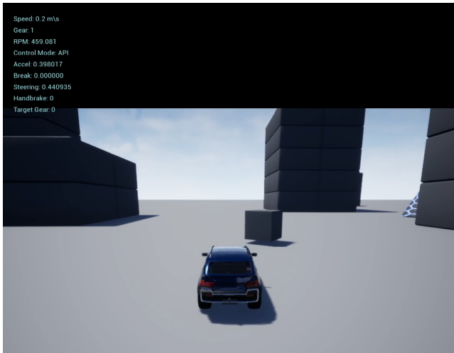
Figure 4: Sample decision in Complex map. Steer and acceleration values are 0.398 and 0.44, respectively
