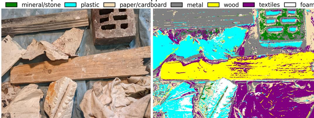
Figure 5. **Left:** RGB picture of a captured scene in lab setting. **Right:** Classified scene.
