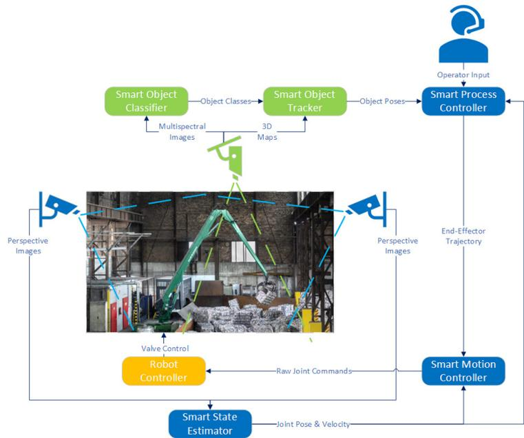
Figure 1. Concept developed in SmartRecycling-UP project for control of heavy hydraulic machines.
