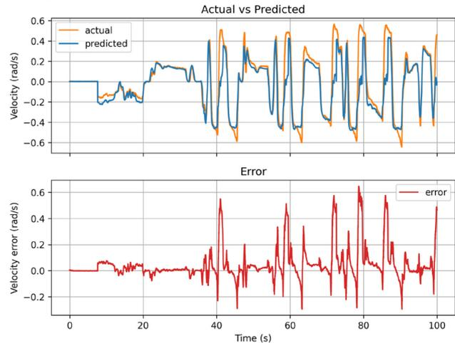
Figure 10. Performance of learned network for prediction of motion with test data.
