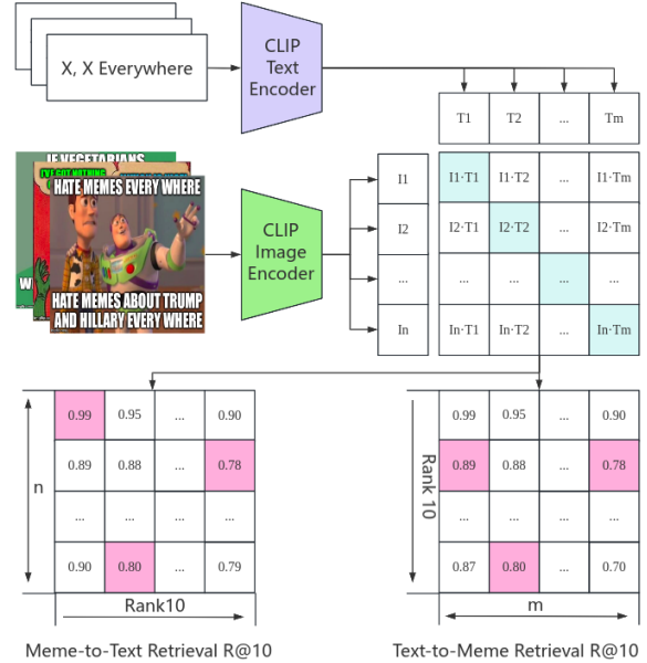
Figure 1: Diagram of meme-text retrieval, illustrated with Recall@10 for clarity, where n and m represent the numbers of memes and texts respectively. Meme and text embeddings are normalized to compute cosine similarities. The light blue cells indicate true matches in the similarity matrix, while the pink cells highlight true matches within the ranked lists.
