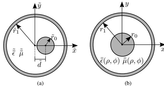
Fig. 1: (a) Cross-section  $\tilde{\Omega}$  of an eccentric coaxial waveguide invariant along the axial direction. (b) Cross-section  $\Omega$  of the mapped concentric coaxial waveguide.
