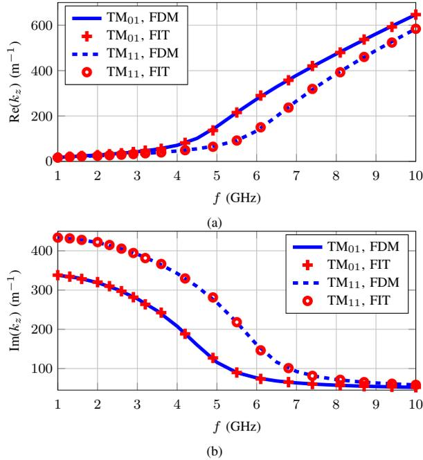
Fig. 5: Axial wavenumbers for the  $TM_{01}$  and  $TM_{11}$  modes as a function of frequency.
