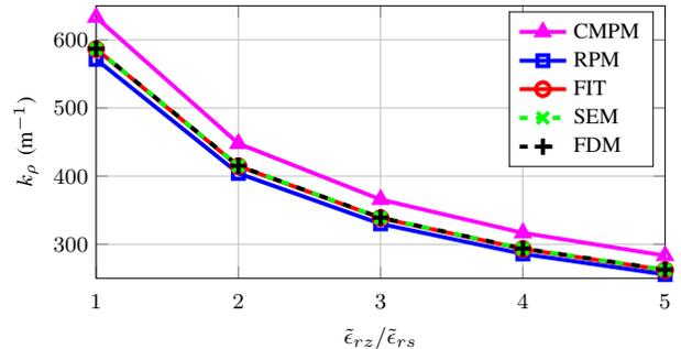
Fig. 4: Radial wavenumbers for the  $\text{TM}_{01}$  mode as a function of the anisotropic permittivity ratio  $\tilde{\epsilon}_{rz}/\tilde{\epsilon}_{rs}$ , with  $\tilde{\epsilon}_{rs} = 1$ .
