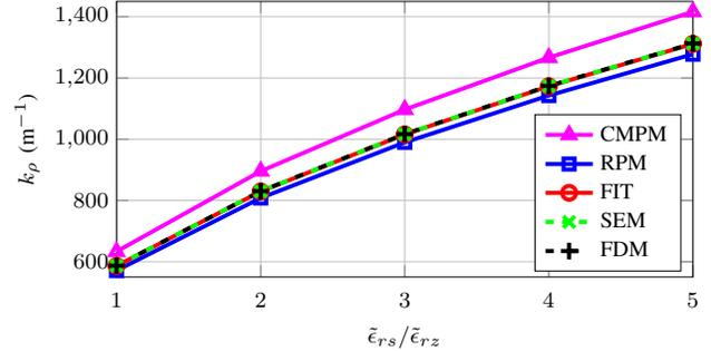
Fig. 3: Radial wavenumbers for the  $\text{TM}_{01}$  mode as a function of the anisotropic permittivity ratio  $\tilde{\epsilon}_{rs}/\tilde{\epsilon}_{rz}$ , with  $\tilde{\epsilon}_{rz} = 1$ .
