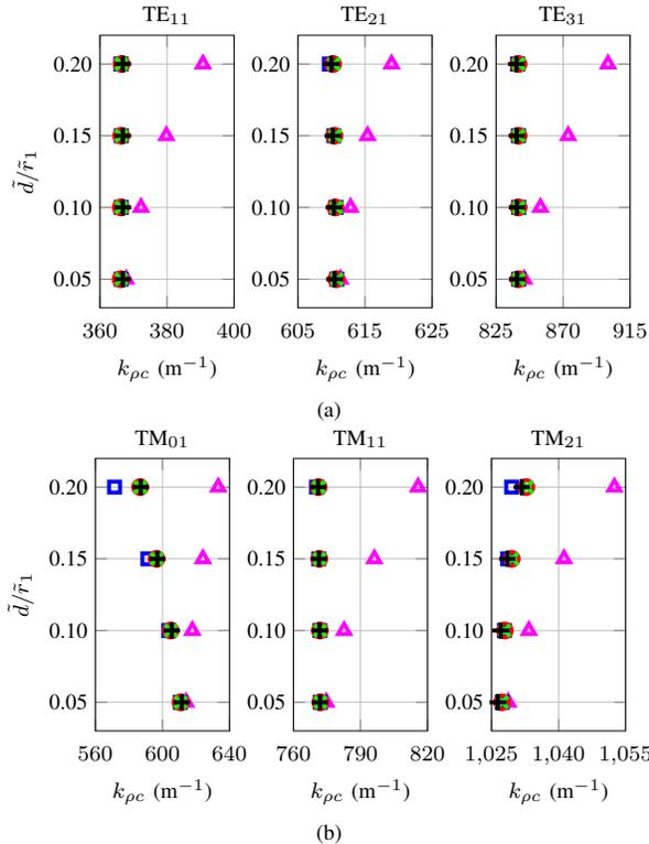
Fig. 2: Radial wavenumbers for (a) TE and (b) TM modes as a function of the normalized distance  $\tilde{d}/\tilde{r}_1$  get by CMPM ( $\triangle$ ), by RPM ( $\square$ ), by FEM ( $\circ$ ), by SEM ( $\times$ ), and by FDM ( $+$ ).
