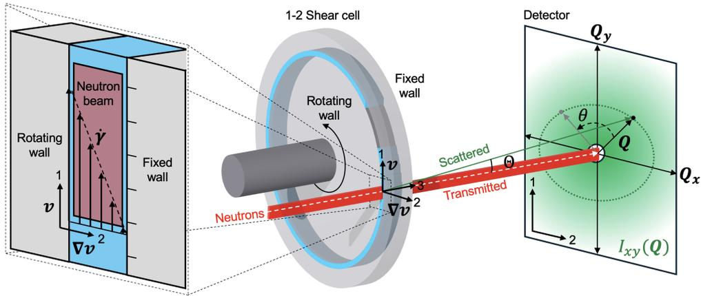
Figure 2: Schematic of the SANS experiment conducted under Couette geometry. The directions of flow ( $v$ ), velocity gradient ( $\nabla v$ ), and vorticity ( $\nabla \times v$ ) are indicated as 1, 2, and 3, respectively. Two-dimensional SANS spectra were acquired in the flow-velocity gradient plane (1-2 or  $\nabla v-v$ ).
