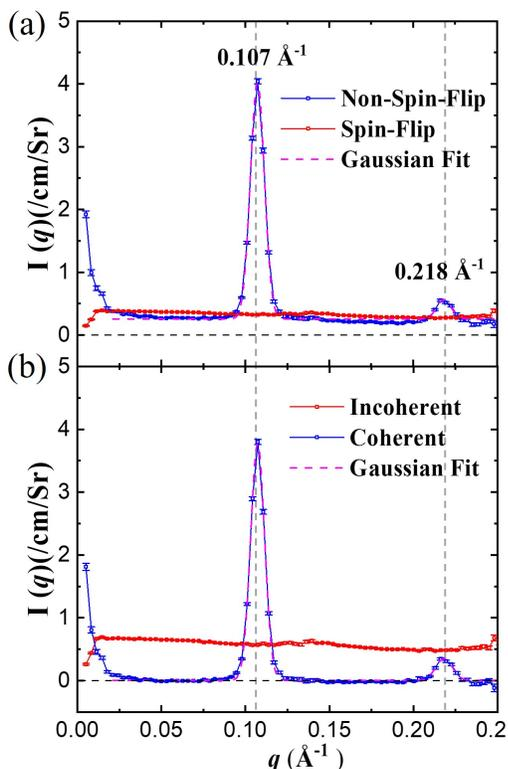
FIG. 5: Radially averaged scattering data on an absolute scale after PASANS correction on both #2 and #3 detectors. Corrected spin-flip and non-spin-flip scattering curves are indicated as empty blue and red squares in (a). Separated nuclear spin incoherent and coherent scattering curves shown in red and blue empty squares in (b). Two diffraction peaks in the non-spin-flip scattering and nuclear coherent scattering curves are fitted using a Gaussian equation, depicted as a magenta dashed line.
