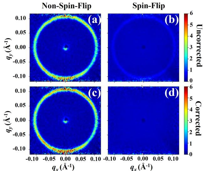
FIG. 4: Diffraction patterns of AgBE powder collected by #3 detectors. (a) and (b): Non-spin-flip ( $\sigma_{-}^s(q)$ ) and spin-flip ( $\sigma_{+}^s(q)$ ) scattering patterns after absolute intensity normalization, except the PASANS correction. (c) and (d): PASANS corrected scattering patterns.
