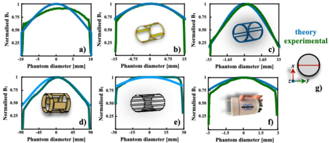
Fig. 4. Comparison of uniformity plots generated from the phantom image data in Fig. 3 and eq. (1) at magnetic field strengths of 4 T (d), 7 T (b, c, e, f), and 15.2 T (a). All profiles were acquired along the red line shown in (g).
