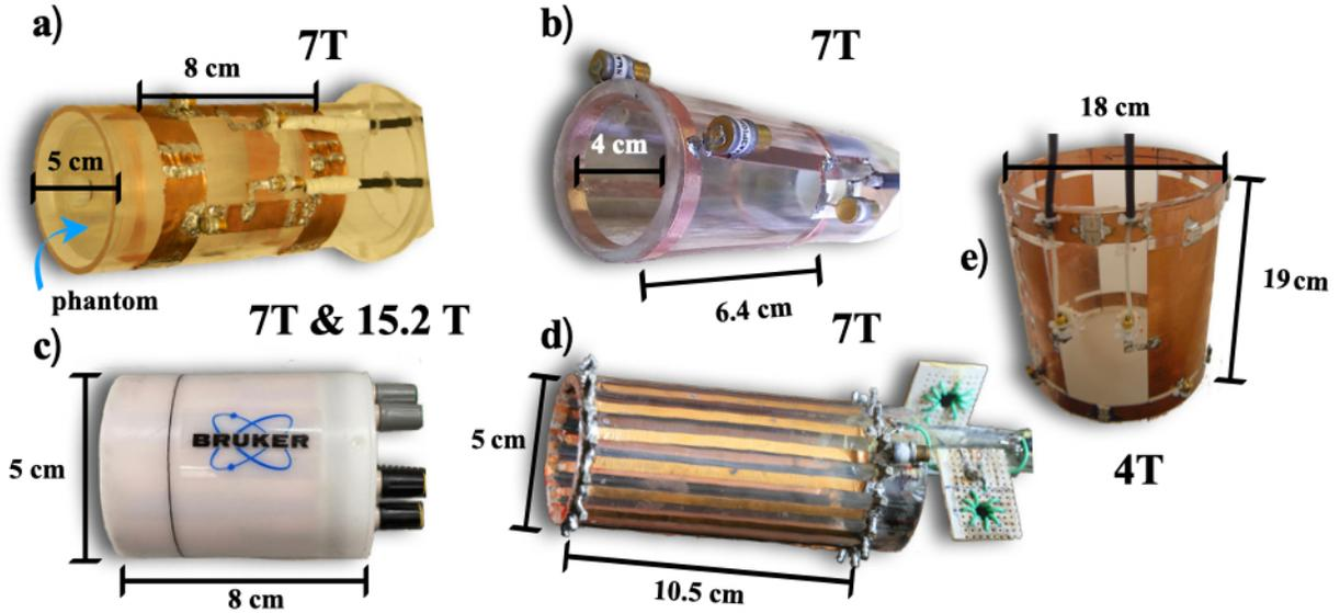
Figure 1. Photographs of the vendor-provided (c) and in-house (a, b, d, e) birdcage coils are shown, highlighting their dimensions for comparison.
