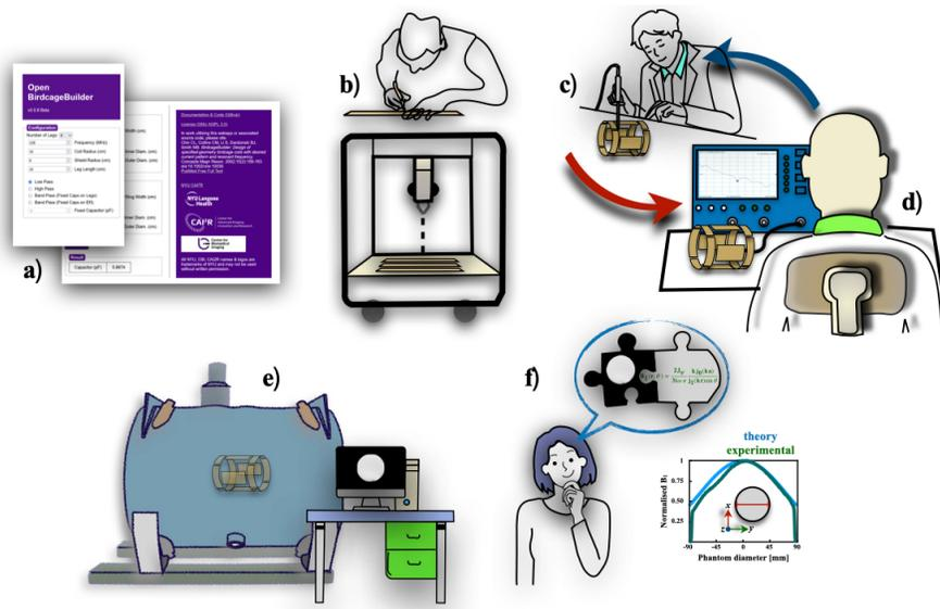
Fig. 2. Schematic of BC coil development process: a) Calculation of passive component values for resonant frequency and  $50 \Omega$  impedance [?]. b) Construction of the prototype using copper sheet or 3D printing. c) and d) Iterative tuning for  $50 \Omega$  impedance matching. e) Image acquisition. f) Validation through comparison of experimental and theoretical results.
