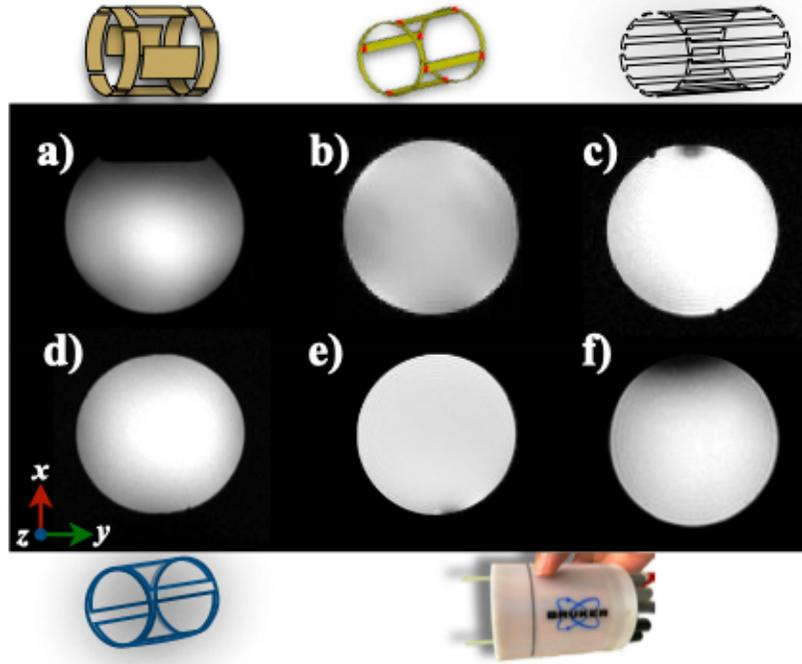
Fig 4. Phantom images acquired using the in-house and vendor-provided birdcage (BC) coils: a) 4 T, b)-e) 7 T, and f) 15.2 T, with the MRI systems described in Fig. 3.
