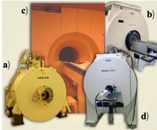
Figure 3. MRI systems used to experimentally test the in-house and vendor-provided birdcage (BC) coils at different resonant frequencies: a) 7 T imager (Agilent, Santa Clara, CA), b) 7 T imager and d) 15.2 T imager (Bruker BioSpin MRI, GmbH, Ettlingen, Germany), c) 4 T imager (Varian, Inc., Palo Alto, CA, USA and Siemens Healthineers AG, Erlangen, Germany).
