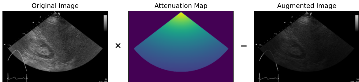
Figure 4: An example of the depth attenuation augmentation on the AUL dataset with a maximum attenuation ( \lambda ) of 0 and attenuation rate ( \mu ) of 1.5.
