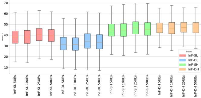
Fig. 4: SINR Distribution by Profile and No. of UEs in uplink transmission
