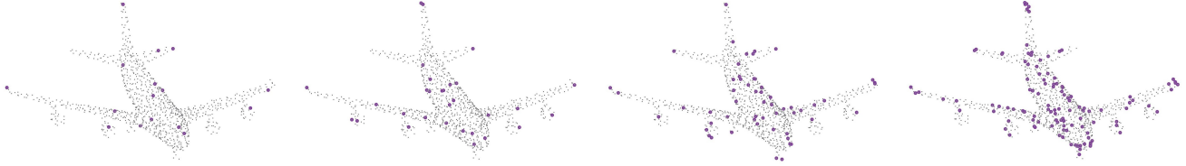
Figure 9. The sampled points through the MorphoSkel3D method, together with the surface points of an airplane example. From left to right the four ratios: 16, 32, 64 and 128 sampled points.
