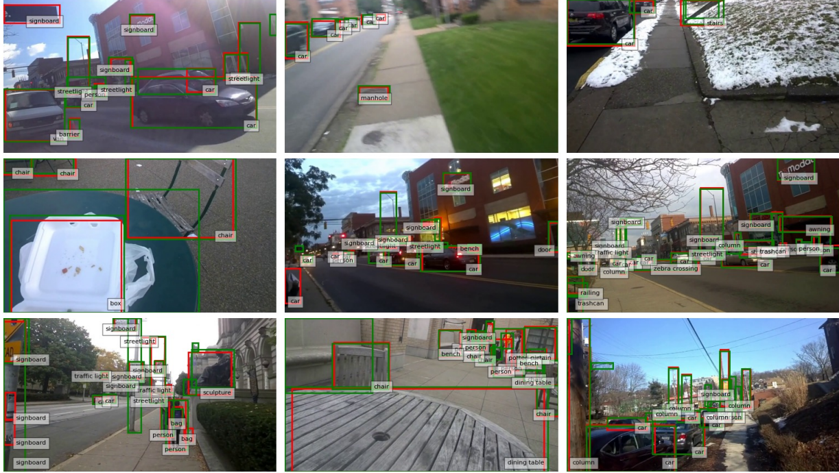
Figure 4: Visualization of object detection results on the OAK validation set. The Memory Storyboard model is trained on KrishnaCam and fine-tuned on the OAK training set. Red boxes show the predictions and the green boxes are ground truth bounding boxes.
