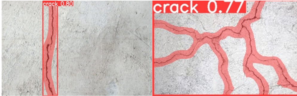
Figure 9: Testing the Accuracy of the Model with a Random Photo Taken from the Internet
