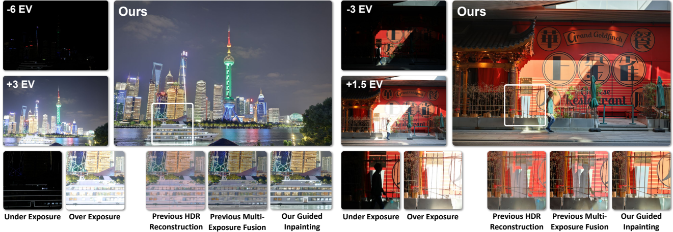
Figure 1. Comparing our guided inpainting HDR imaging method with a state-of-the-art HDR reconstruction [26] and multi-exposure fusion [49] methods. Both scenes are selected from our captured new real-world benchmark. Left : night cityscape with large exposure difference. Right : afternoon street with motion-induced occlusion. Previous methods struggle to handle these scenes. By modeling HDR as inpainting problem, our method can produce visually appealing results without ghosting artifacts in these challenging scenes.
