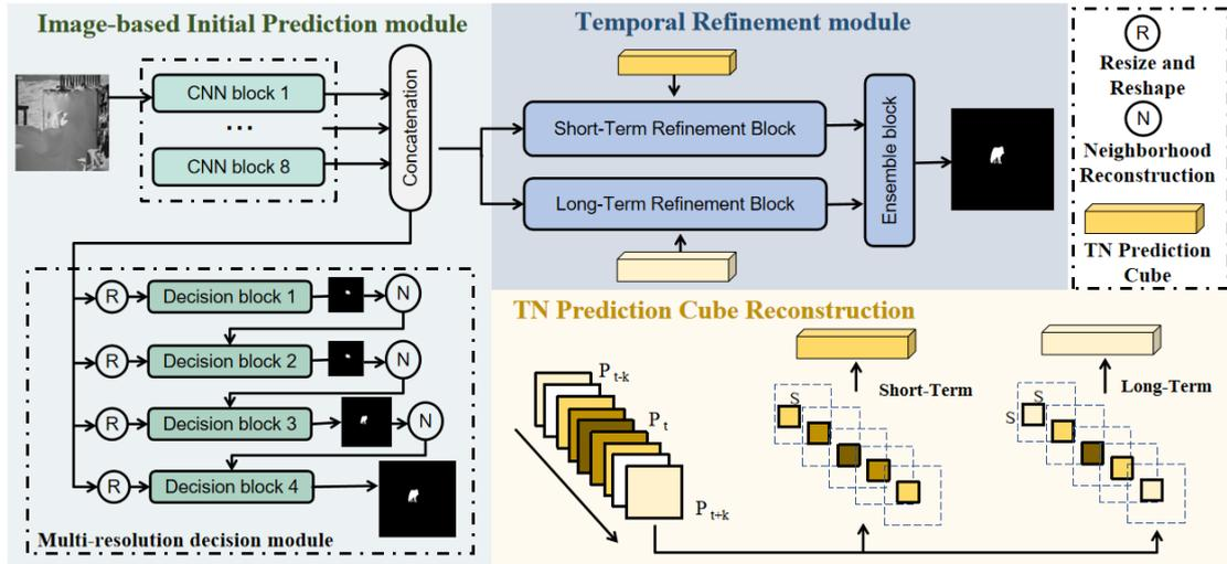
Fig. 1. The system diagram of the proposed green video camouflaged object detection method (GreenVCOD).
