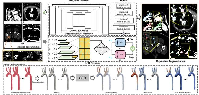
**Fig. 1.** The top shows the flow diagram of LoGB-Net. The Bayesian segmentation results’ blue, red, and green lines represent the segmentation’s upper bound, mean, and lower bound. The bottom displays the application of UQ in aorta segmentation for downstream tasks, such as CFD simulation.
