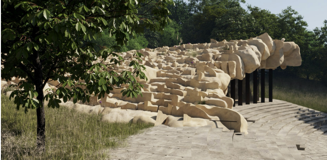
Figure 4: Probobli Boboli : Alternative architectural forms are autogenerated according to a recipe of probable stones - analysed, positioned and connected to form surfaces with continuous water drainage paths. See films at [24].
