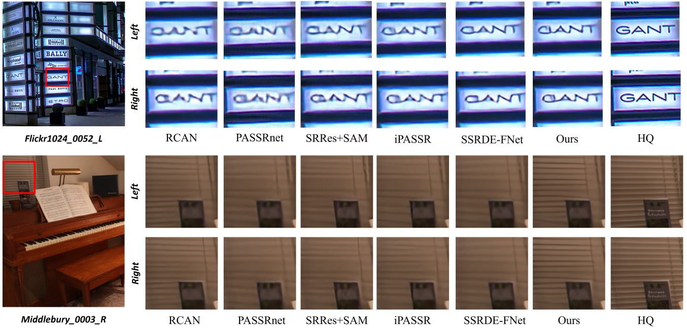
Figure 4: Visual comparisons for \times 4 SR by different methods on Flickr1024 and Middlebury dataset.
