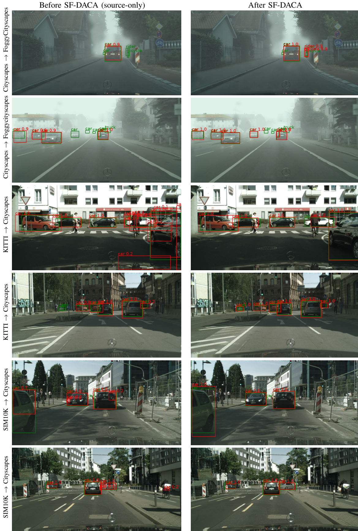
Fig. 2. Qualitative examples from the C→F (top 2 rows), K→C (middle 2 rows) and S→C (bottom 2 rows) adaptation scenarios. Detections of source-pretrained model (left) versus predictions of target-adapted model via SF-DACA (right). Green bounding boxes refer to the groundtruth, and red ones refer to the detections. Detected object class and confidence are provided on the top left of each instance. Best viewed in color.
