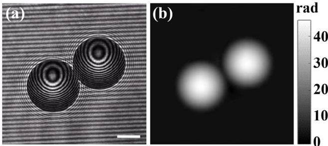
**Figure 12.** Single-shot operation principle demonstration of H2S2MIM involving flowing microbeads: (a) holograms ([Visualization 1](#), 0.5 MB) and (b) unwrapped phase images ([Visualization 2](#), 0.25 MB). Scale bar represents 20  $\mu\text{m}$ . (Movies taken from [81] by permission of OSA).
