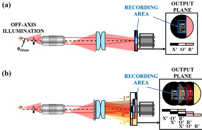
**Figure 4.** Scheme of the S2MIM layout for the case of tilted beam illumination before (a) and after (b) diffraction grating insertion.
