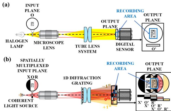
**Figure 1.** Optical scheme of a regular microscope before (a) and after (b) SMIM application, pointing the modifications introduced by SMIM.
