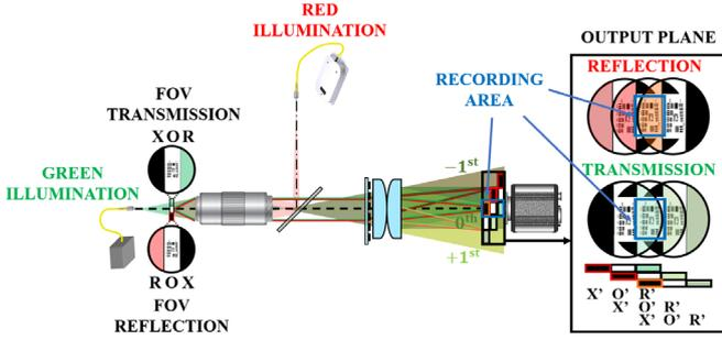
**Figure 6.** Optical scheme and ray tracing of the OV-SMIM approach.
