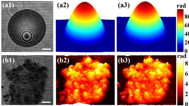
**Figure 11.** Experimental validation of H2S2MIM involving static samples: (a1) and (b1) holograms for the case of a 90  $\mu\text{m}$  sphere and prostate cancer cells, respectively, and (a2)-(b2) and (a3)-(b3) perspective views of unwrapped phase distributions provided by H2S2MIM and by temporal P-S algorithm, respectively. Scale bars represent 20  $\mu\text{m}$ . (Images derived from [81] by permission of OSA).
