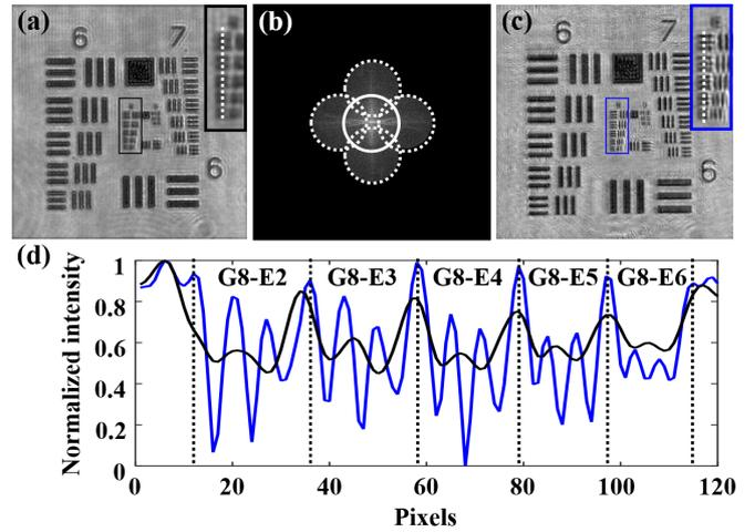
**Figure 5.** Final results of the experimental validation of S2MIM involving a 5X/0.15NA objective and an USAF resolution test target: (a) the low-resolution intensity image provided by conventional SMIM, (b) the SA coming from the addition of the four additional off-axis apertures, (c) the SR image provided by S2MIM, and (d) the plots along the vertical white lines included in (a) and (c). (Images adapted from [78] by permission of OSA).
