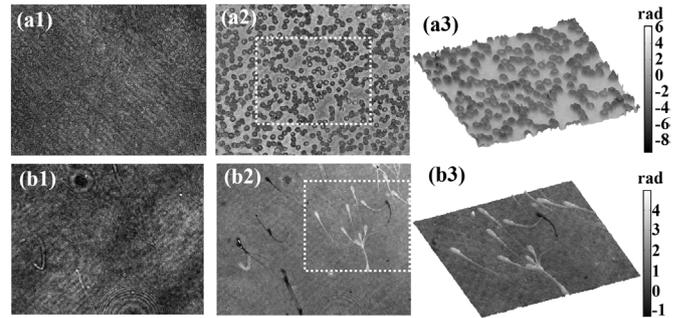
**Figure 3.** Experimental results of conventional SMIM for the cases of RBCs and SSCs using a 20X/0.46NA objective. Column (1) the holograms, column (2) the retrieved phase images, and column (3) the perspective view of unwrapped phase maps of the regions enclosed in the white rectangles in column (2), respectively. (Images derived from Ref. [62] by permission of OSA).
