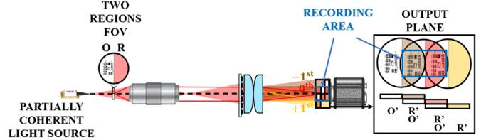
**Figure 9.** Scheme of SMIM approach with partially coherent illumination, where the main changes regarding illumination and FOV spatial multiplexing are identified.
