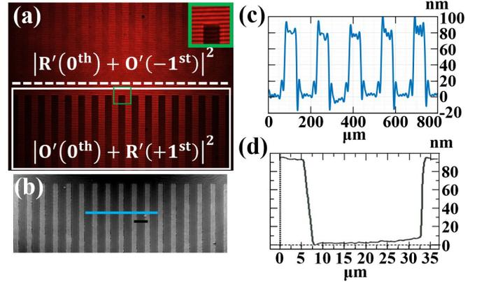
**Figure 7.** Experimental validation of *OV-SMIM* for reflective imaging mode: (a) reflective hologram, (b) retrieved phase distribution of the region enclosed in the solid white rectangle included in (a) after applying temporal P-S method, and (c) and (d) thickness profiles along blue and black lines included in (b) provided by reflective SMIM and AFM, respectively. (Images adapted from [84] by permission of OSA).
