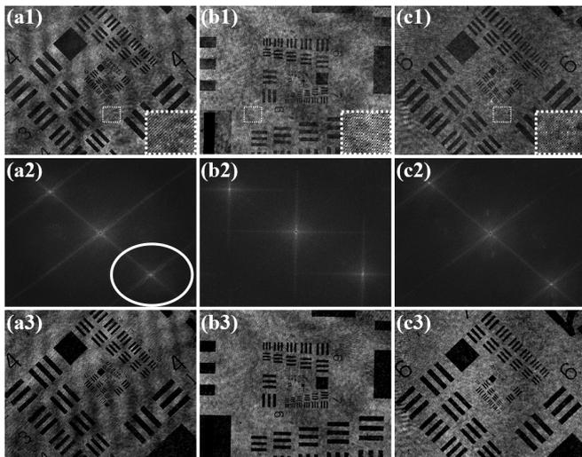
**Figure 2.** Experimental validation of conventional SMIM involving an USAF resolution test target. Columns (a)-(c): results for the 5X, 10X, and 20X lenses, respectively. Rows (1)-(3): holograms, Fourier transforms of the holograms, and retrieved intensity images, respectively. (Images adapted from [62] by permission of OSA).
