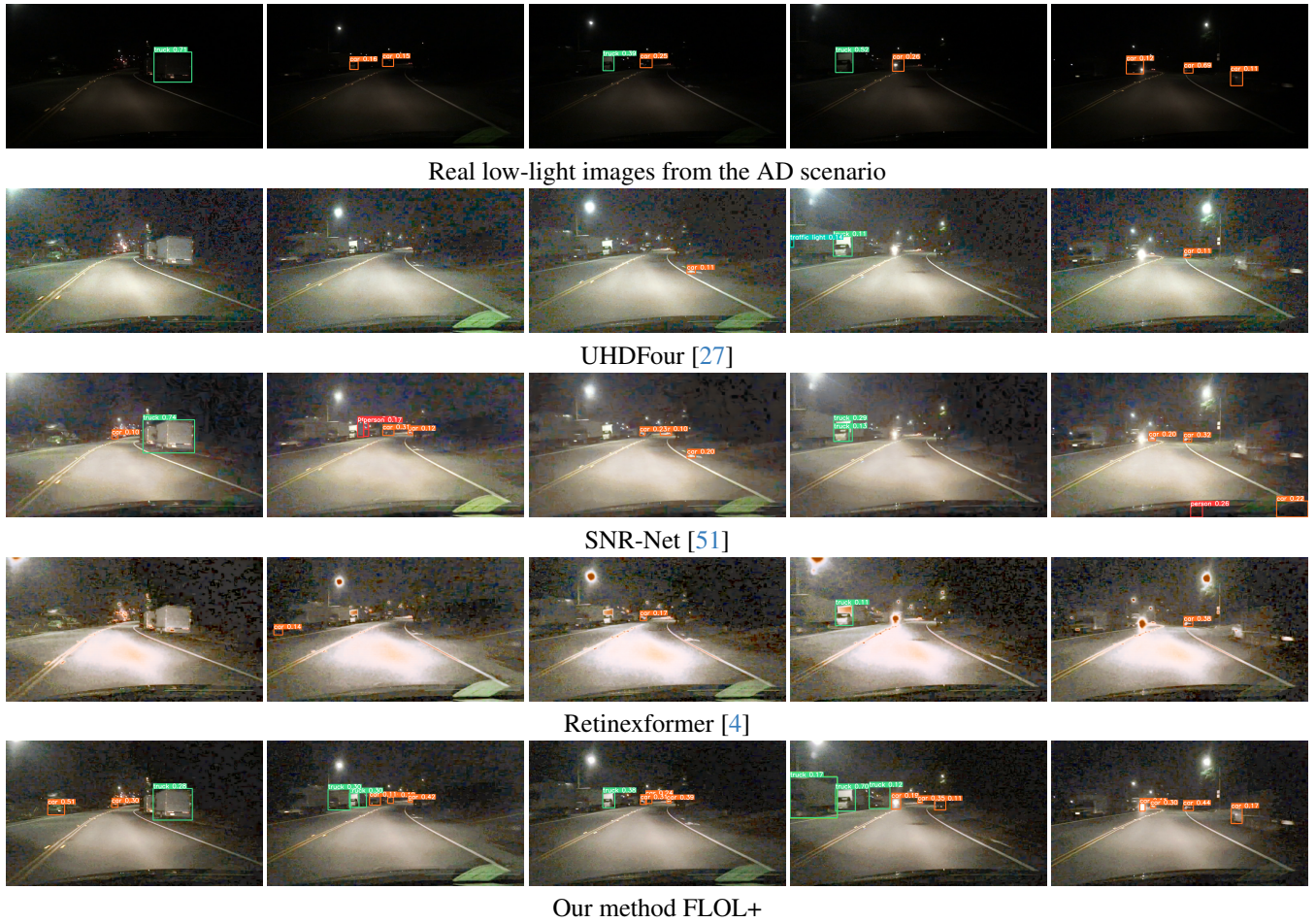
Figure 10. Comparison of qualitative results on the Autonomous Driving Dataset BDD100k [58]. We can observe how the detector YOLOv8 [35] performs best when we use our method for image enhancement.
