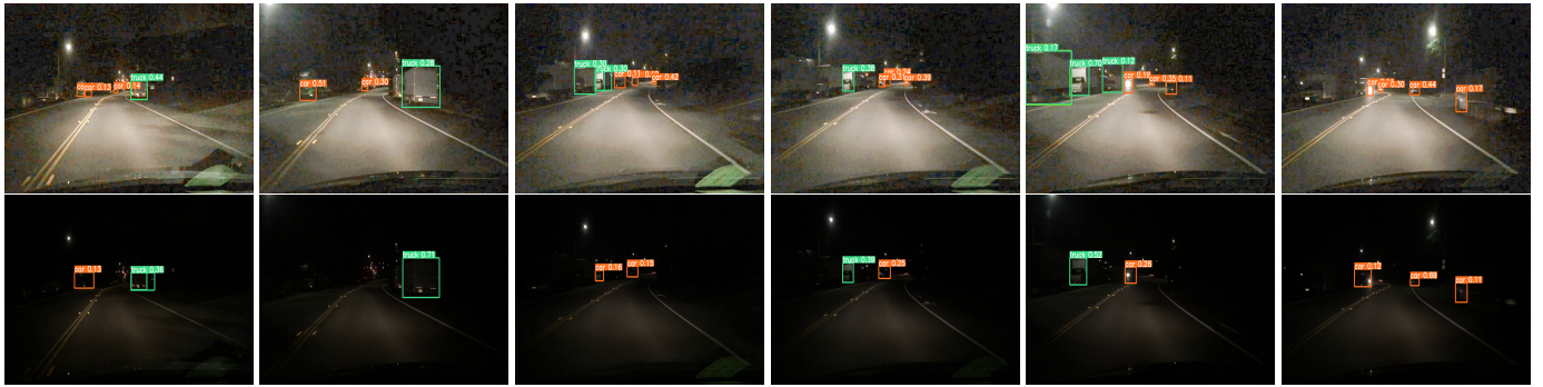
Figure 9. Results of FLOL+ in a sequence of frames belonging to a video from the BDD100k [58] dataset. We run again YOLOv8 in both images (low and high), where green labels correspond to class truck and orange labels correspond to class car. (Zoom in for best view).
