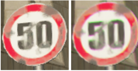
Fig. 9. Pinhole (left) vs. PSF-Filtered Image (right)
