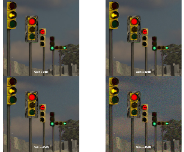
Fig. 13. Traffic Light Image Example with Four Levels on Camera Gain
