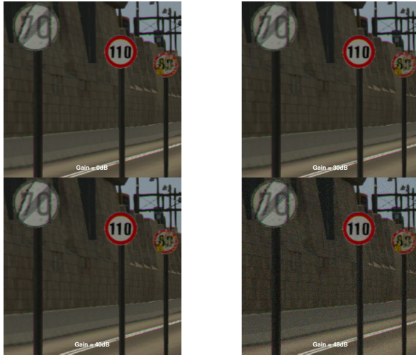
Fig. 12. Speed Sign Image Example with Four Levels on Camera Gain
