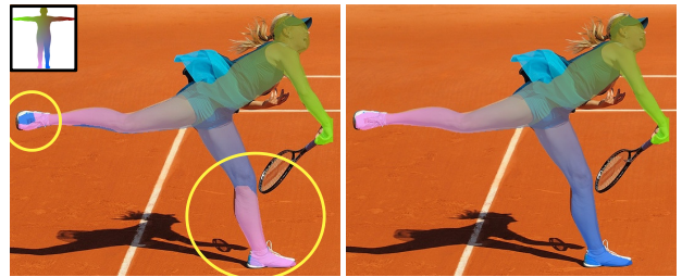
Figure 1. The Continuous Surface Embedding method (CSE) [20] (left) vs. Pose-Constrained CSE (right). The CSE method assigns each pixel of body segmentation to a vertex, and thus UV coordinate, on a canonical body shape mesh. The CSE assigns each pixel independently, leading to artifacts such as limb duplication (yellow circles). PC-CSE uses pose constraints during UV map estimation, producing smoother maps and eliminating artifacts. The UV values at individual pixels are visualized by color coding. The location of a given color on the canonical surface is shown in the inset image at the top left.
