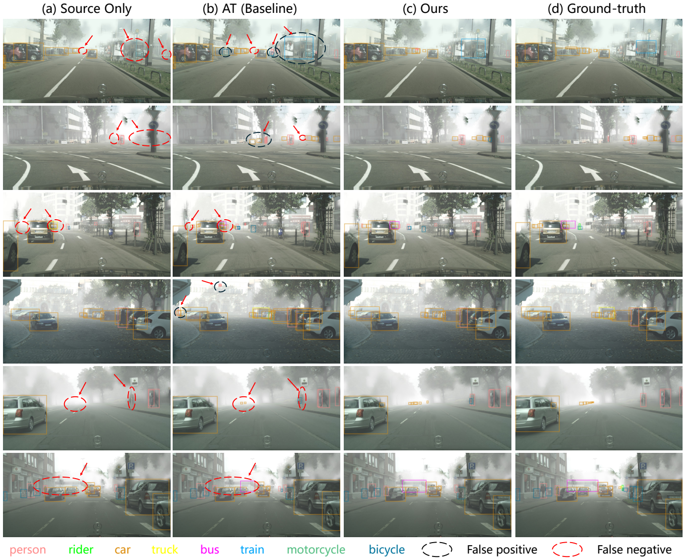
Fig. 6. Qualitative results on the Cityscapes-to-FoggyCityscapes adaptation scenario of (a) the Source Only model, (b) Baseline [14], (c) Ours , and (d) Ground-truth . (Zooming in for best view.)
