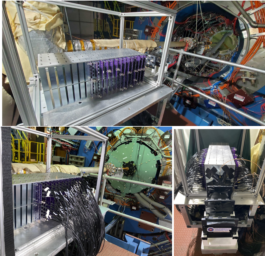
Figure 2. Top: The prototype partially installed on the East Platform of the STAR detector [32] (background). The nominal STAR interaction point is visible in this view, with no detector material obstructing the line of sight between the prototype and the interaction point. Bottom left: Rear view of the fully installed prototype. In this view, the STAR detector is in its nominal configuration, with the STAR Event Plane Detector [33] (green disk) being the only material in the line of sight between the prototype and the interaction point. Bottom right: Front view of the fully installed prototype. The hodoscope detector positioned in front of the prototype was not utilized during the first phase of the experiment presented in this work.
