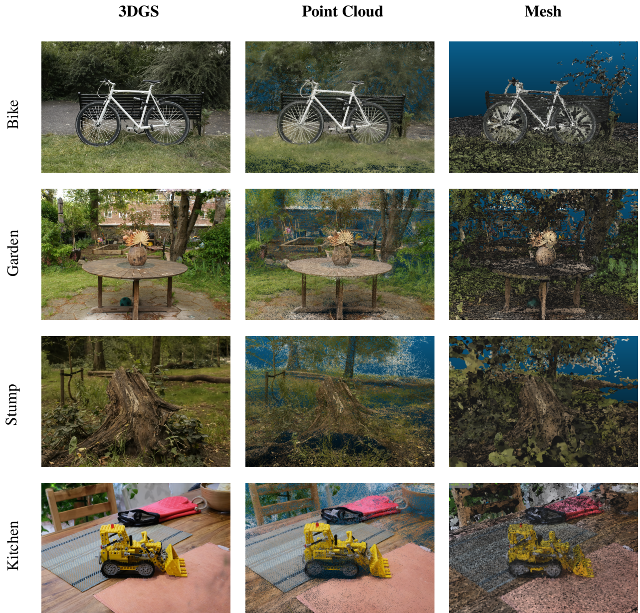
Figure 6: Comparison between the 3DGS, point cloud and mesh representations for four different Mip-NeRF 360 dataset scenes. The point clouds and meshes were generated using 3DGS-to-PC on default arguments, apart from 'clean_pointcloud' was set to true and the 'poisson_depth' was set to 12 (to increase mesh quality). The Bike scene had an bounding box, -5 to 5 in every dimension, implemented only on the mesh, to improve visual clarity of the bike in the image. The 3DGS images were rendered using the official 3D Gaussian Splatting SIBR interactive viewer, while the point cloud and meshes images were generated from the CloudCompare viewer.
