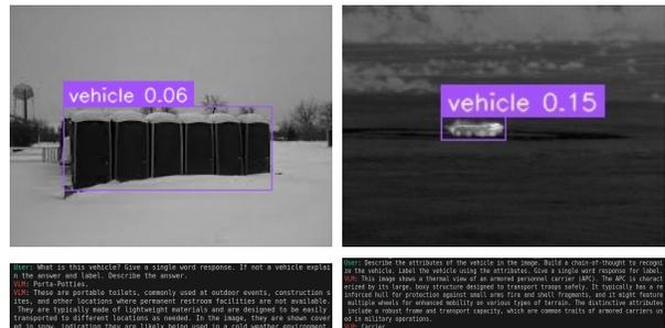
Fig. 5. The pipeline can be used to remove false positives (left image) produced by the detector. The Chain-of-thought recognition on the thermal image illustrates the attributes used to label the object.
