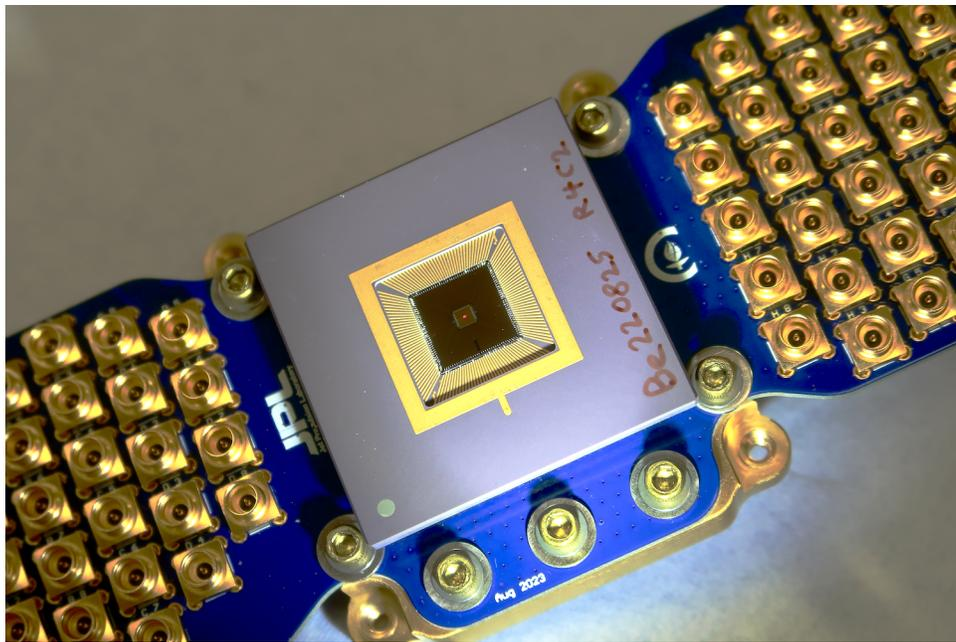
Fig. 9. SNSPD array packaged in a pin grid array (PGA) chip carrier.
