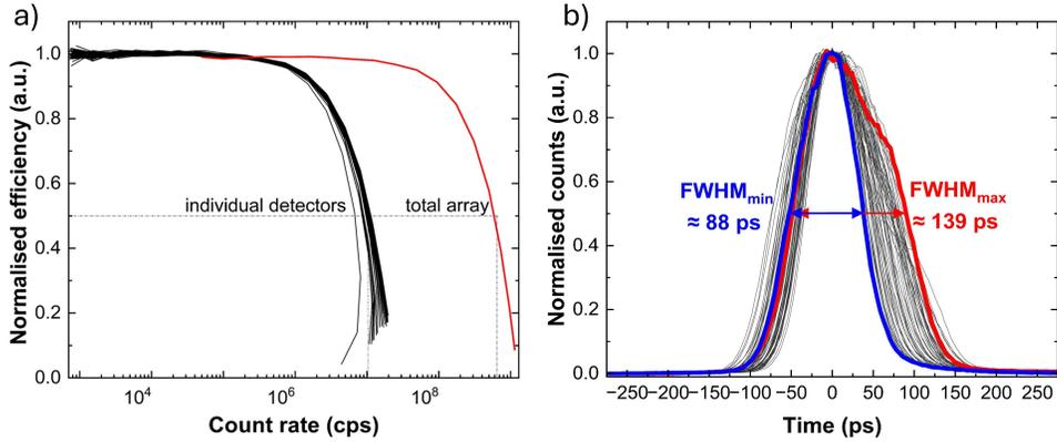
Fig. 3. a) Normalised efficiency of the 64 pixel SNSPD array versus measured count rate. The intersecting dashed lines indicate the MCR at the 3-dB compression point for the total array and also in the centre of the range of individual pixels. b) Temporal jitter histograms of all 64 pixel in the SNSPD array. The highlighted red and blue lines represent the from 2 individual pixels which exhibited the minimum (blue) and maximum (red) FWHM jitter values.
