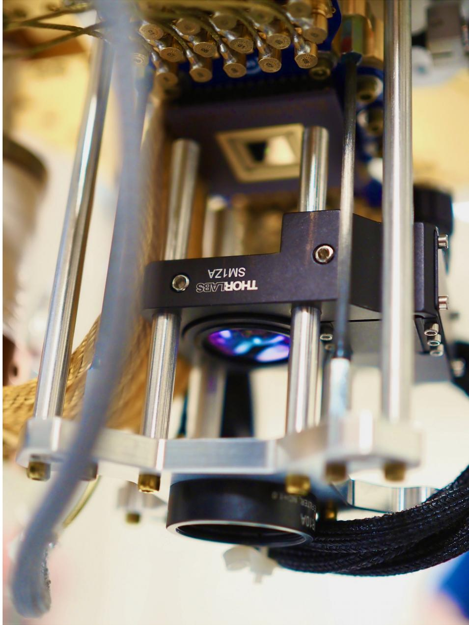
Fig. 8. SNSPD array and chip carrier mounted onto the cryostat 1K stage with the final imaging lens mounted on an optical cage system.
