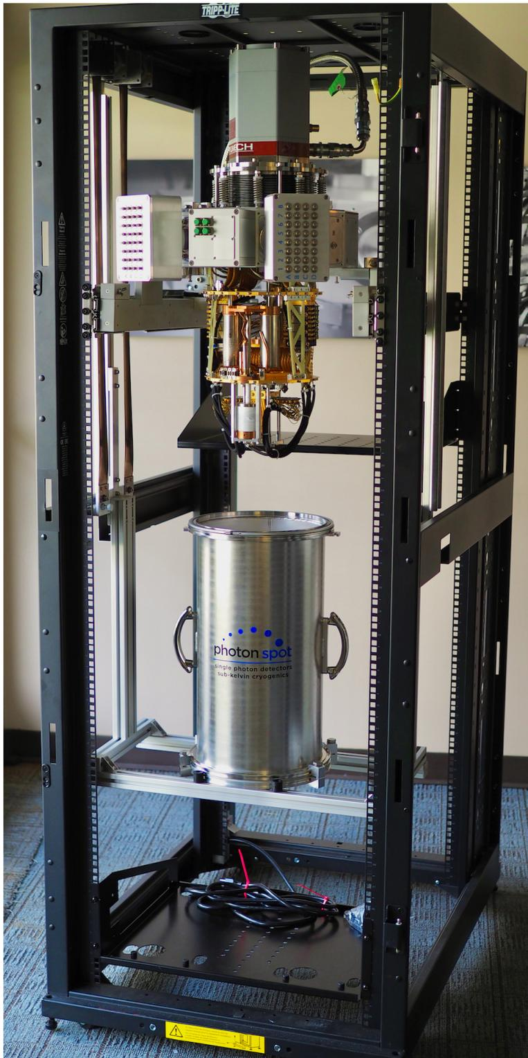
Fig. 6. Lowered cryostat housing and rack-mounted lowering mechanism.
