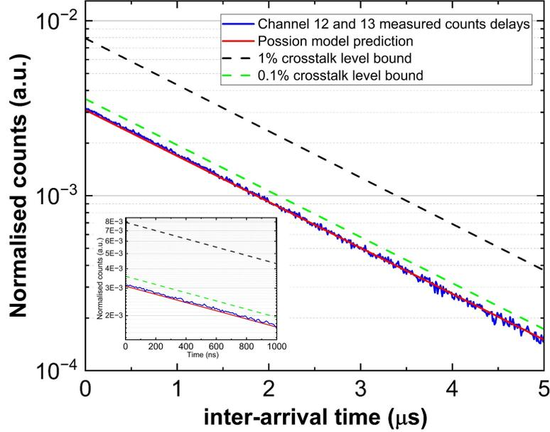
Fig. 4. Probability of detecting an event on Channel 13 following an event on Channel 12 as a function of inter-arrival time. Blue solid line: measured values. Red solid line: un-correlated Poisson model prediction. Black and green dashed lines: upper limit of correlations with 1% and 0.1% crosstalk respectively. The inset graph shows a zoomed in view on the timescale of 0 – 1  $\mu$ s.
