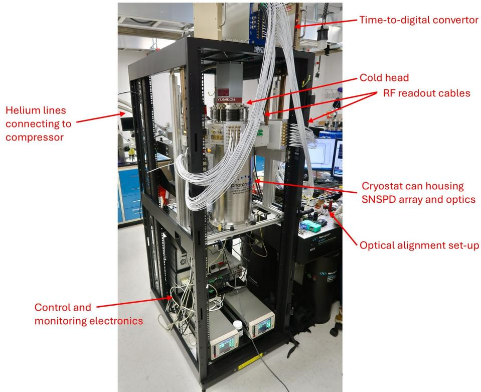
Fig. 5. Photograph of rack containing the SNSPD camera cryostat, cryogenic control instruments, SNSPD electronics modules, and time-tagging electronics.
