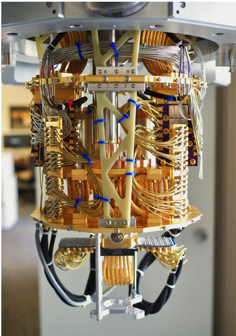
Fig. 7. Cryostat internal components including the cryogenic amplifiers.
