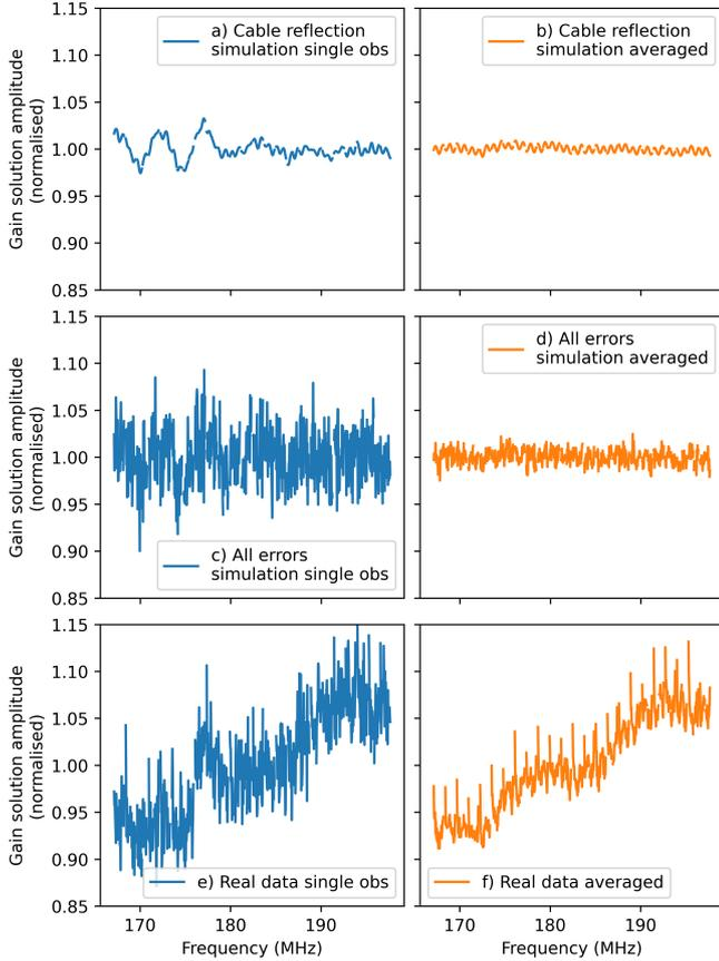
**Figure 9.** Calibration amplitudes showing the effects of averaging calibration solutions over 15 observations. Calibrations for a single tile are shown; other tiles show similar behaviours. Left column shows a single observation, right the average over 15 observations. Top row shows the simulation only containing cable reflection errors; middle row shows the simulation containing all instrumental errors; bottom shows real data.
