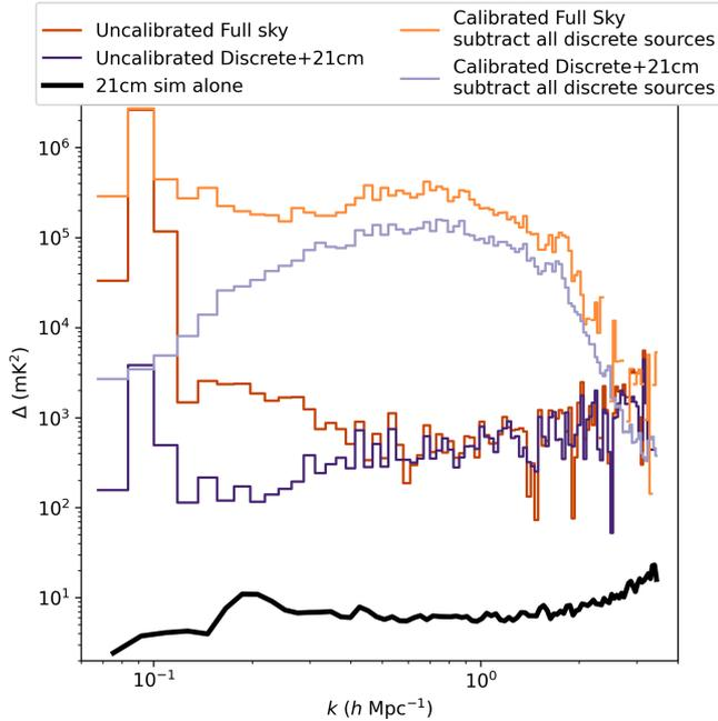
**Figure 5.** 1D PS depicting data from a single zenith EoR0 observation, showing the effects of calibration on leakage into the window. Note that the dark purple and brown lines showing uncalibrated simulations are colour-coded to lines showing the same simulations in Figures 3 and 4, for easy comparison.
