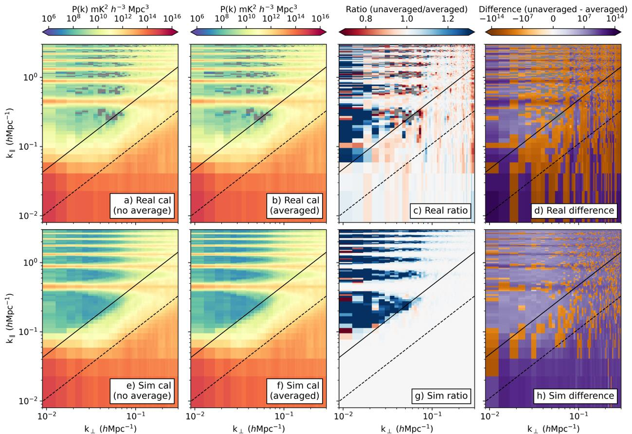
**Figure 10.** Effects of averaging calibration solutions over 15 observations for real data (top row) and simulated data (bottom row). The data in the simulation contain both discrete and diffuse sky models, but do not contain noise, in an attempt to better reveal any systematic bias involved in averaging. The calibration solutions applied to the simulation were derived from a simulation that did contain noise however, so the effects of noise are captured in the calibration solutions.
