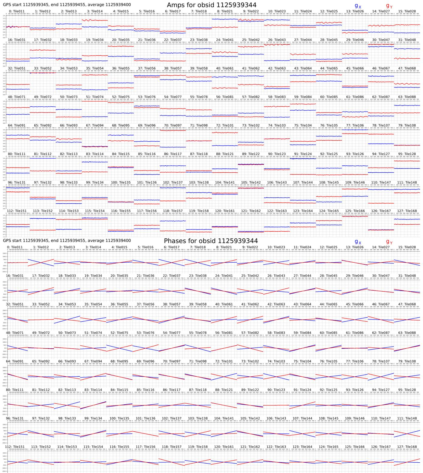
**Figure 11.** Calibration gain amplitudes and phases from a simulated two minute snapshot. These demonstrate the constant gain and flat phase slopes added to the simulation. The underlying simulation was of both the diffuse and discrete sky models, and only contained gain errors with no other instrumental effects. Calibration was performed using 10,000 sources through `hyperdrive`. Any spectral structure in the amplitudes comes from the incomplete sky model rather than injected gains.
