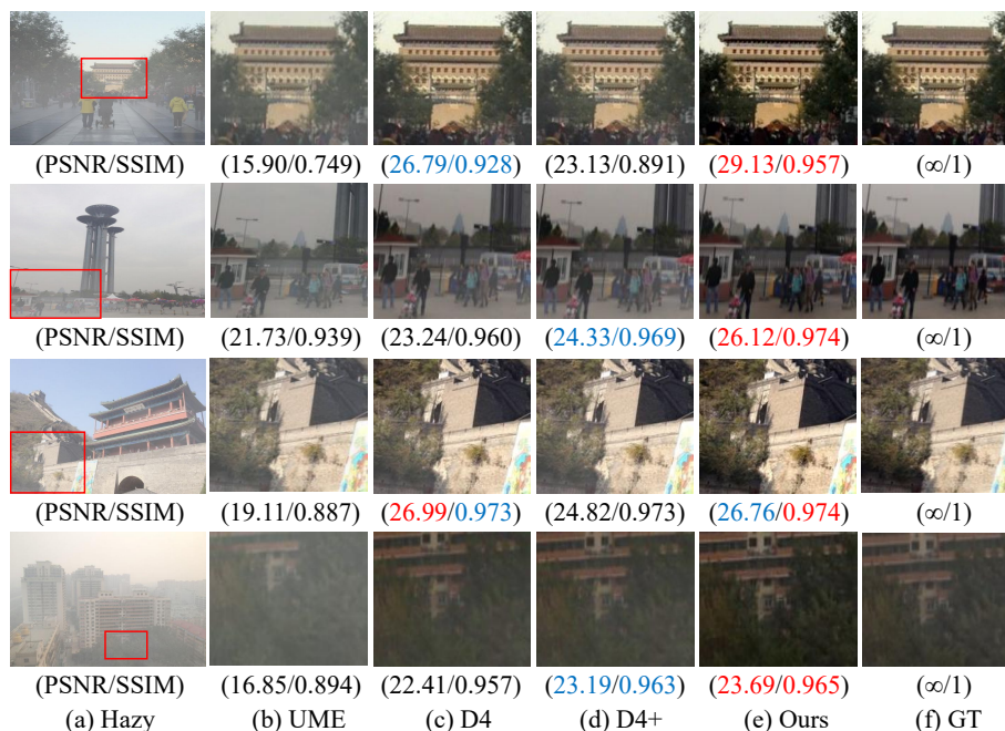
Figure 6: Visual comparison of haze removal on samples from the SOTS-outdoor dataset. It can be seen that, both in terms of visualization and metrics, our method performs the best. The red and blue colors are used to indicate the 1 st and 2 nd ranks, respectively.
