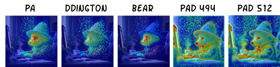
Figure 7: Attention maps for FLUX diffusion show strong alignment between prompt tokens and semantically relevant image tokens. These maps also reveal high attention for padding tokens with the main objects in the image.
